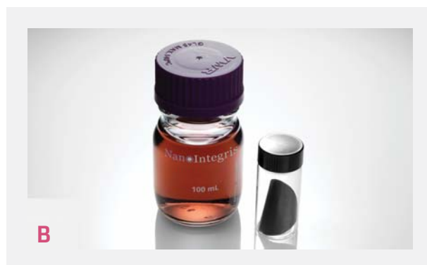
Figure 1. A. 1 mg of metallic IsoNanotubes in solution and 10 mg of metallic IsoNanotubes powder. B. 1 mg of semiconducting IsoNanotubes in solution and 10 mg of semiconducting IsoNanotubes powder. C. 25 mg of PureTubes in solution and 25 mg of PureTubes powder.
